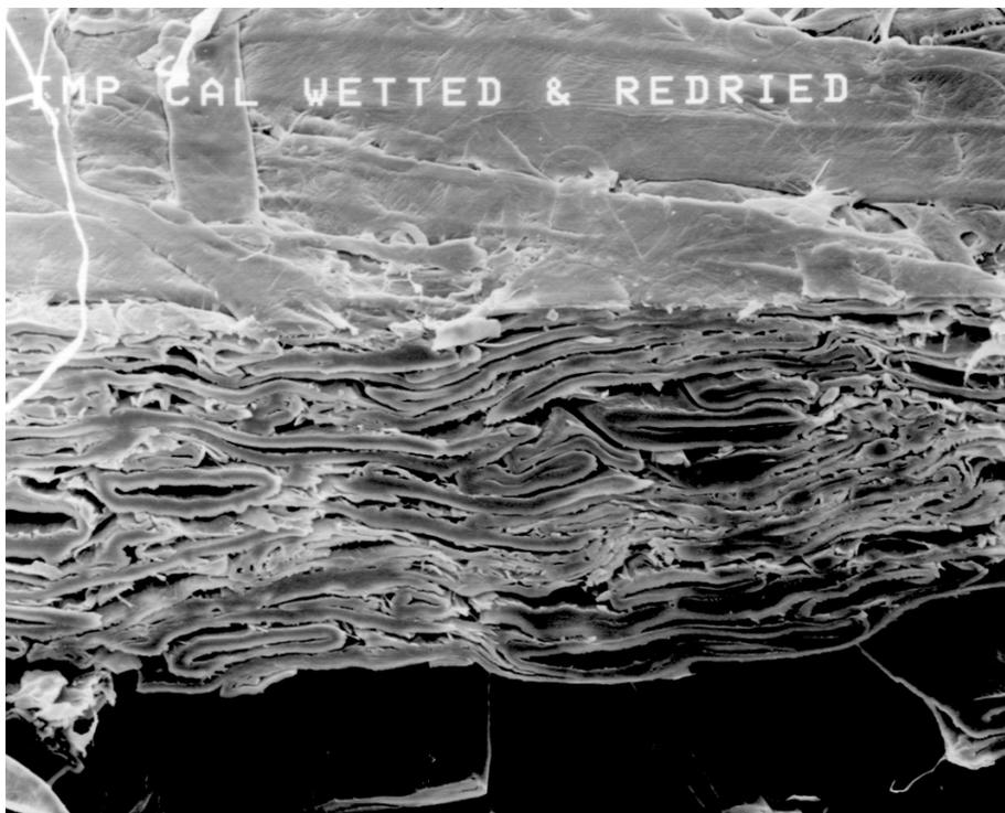
Photo 4 SEM image of calendered TMP sheet wetted and redried.
