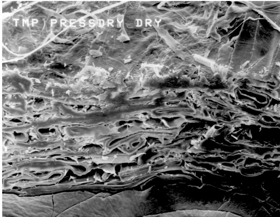
Photo 1 SEM image of press-dried TMP sheet. Top side was
