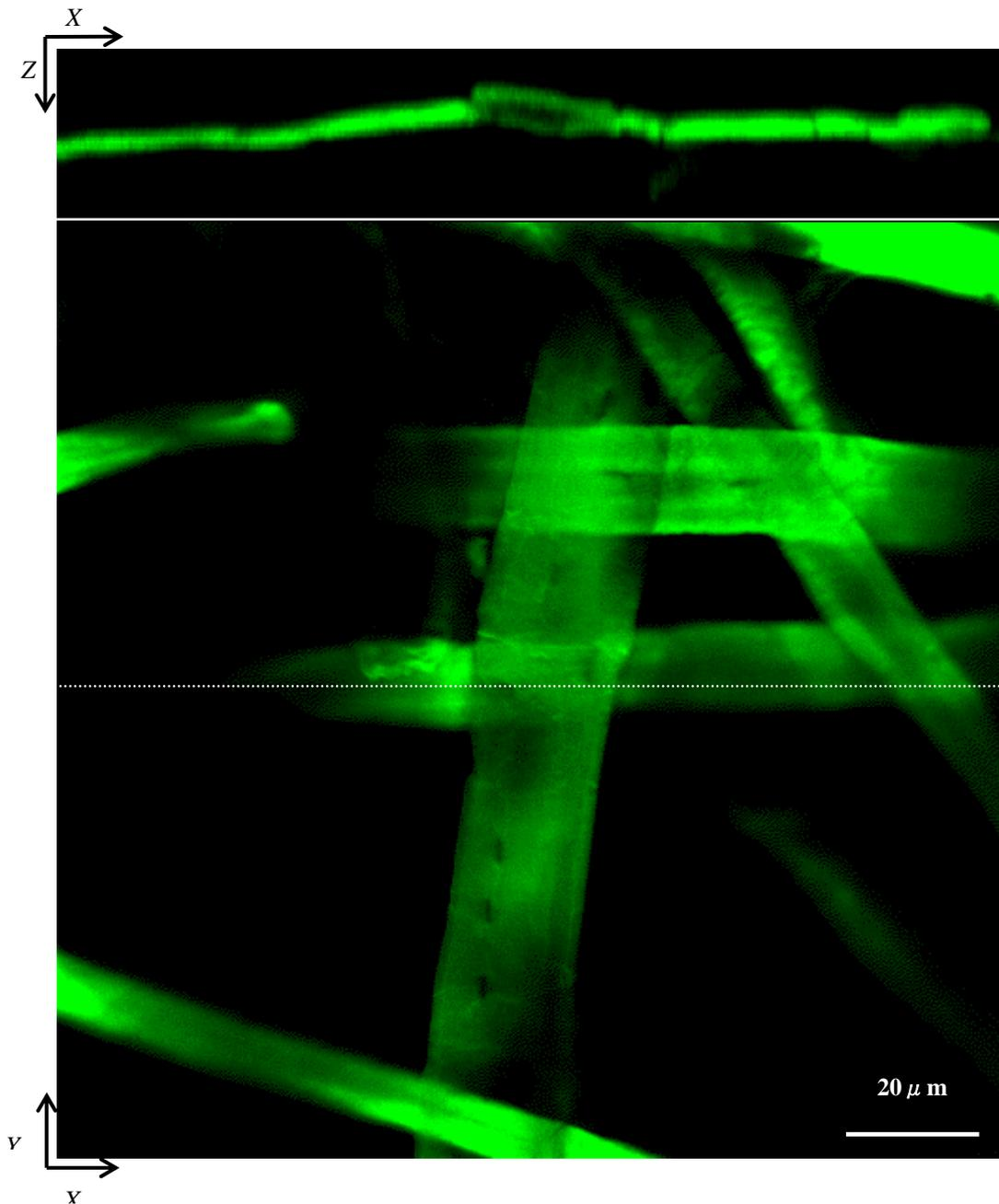
Fig. 8. CLSM XZ-sectioned micrograph (top) along the dotted white line in XY-micrograph (bottom) shows an un-bonded area at the interfiber crossing of dried fiber of post-R4 slurry.
