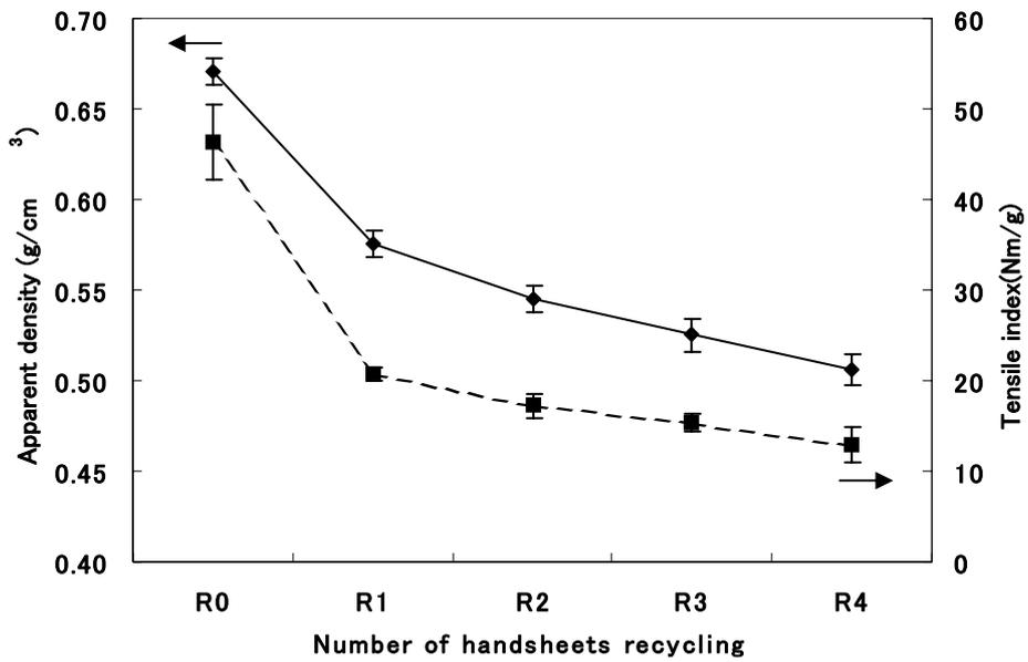
Fig. 1. Decrease in apparent density and tensile index of HBKP handsheets due to the recycling treatment. A pair of bars denotes a range of 95% confidence level.
