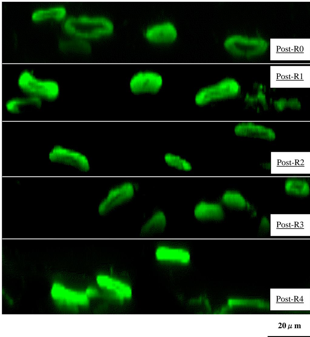
Fig. 5. CLSM micrographs of HBKP fiber (wet) cross-sections show the stepwise effect of recycling treatment on the re-swelling ability.
