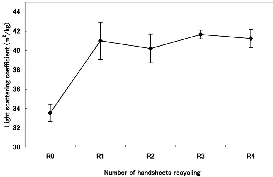
Fig. 9. The increase in light scattering coefficient of recycled HBKP handsheets due to the recycling treatment. A pair of bars denotes a range of 95% confidence level.
