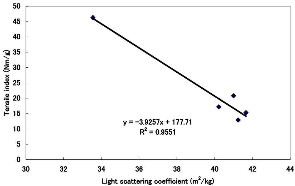
Fig. 10. Relationship between light scattering coefficient and tensile index of HBKP handsheets.
