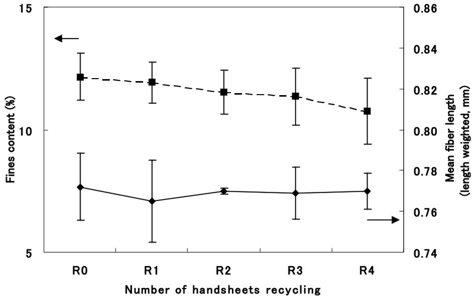
Fig. 4. Fines content and mean fiber length of post-R0 to R4 slurries. A pair of bars denotes a range of 95% confidence level.
