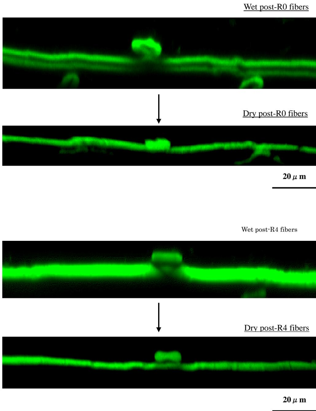
Fig. 7. CLSM micrographs of HBKP fiber cross-sections at the interfiber crossings show the conformability of wet-swollen fibers of post-R0 slurry is superior, for promoting the good interfiber contact in the dry state, to that of wet-collapsed fibers of post-R4 slurry.
