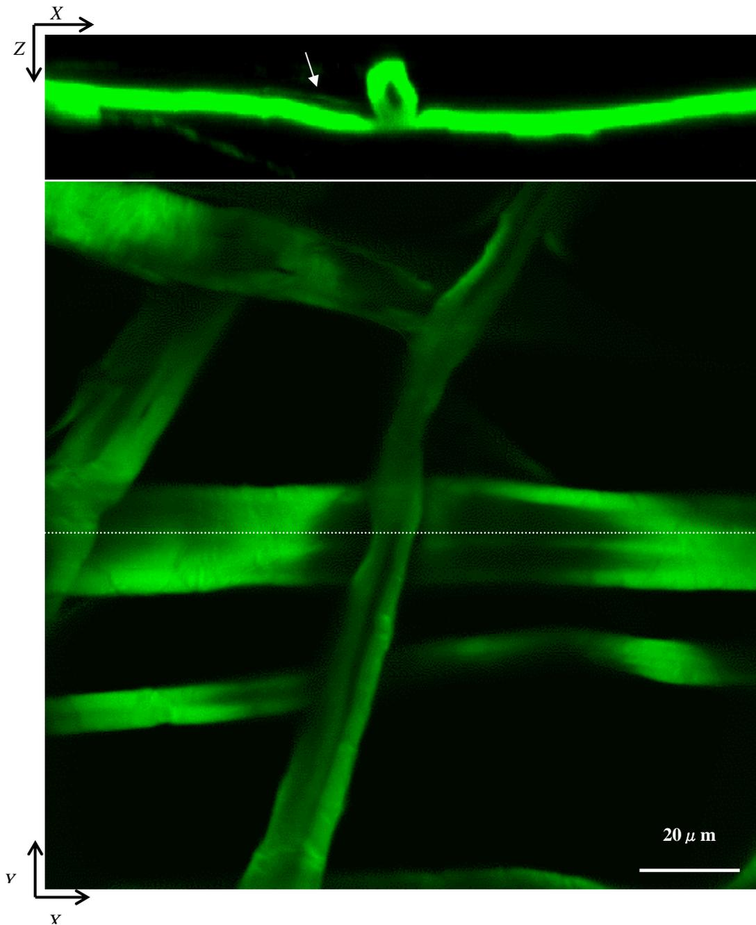
Fig. 3. CLSM XZ-sectioned micrograph (top) along the dotted white line in XY-micrograph (bottom) shows a thin layer of fines (arrowed) covering a fiber surface of post-R0 slurry surface in the dry state at the potentially interfiber crossing as a kind of strengthening material.
