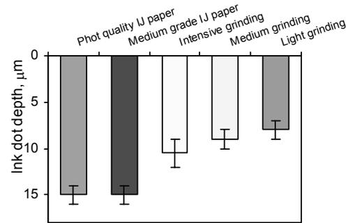
Fig. 5 Ink penetration depth for trial ink-jet papers coated with ground calcium carbonate pigments compared to those for commercial ink-jet papers
