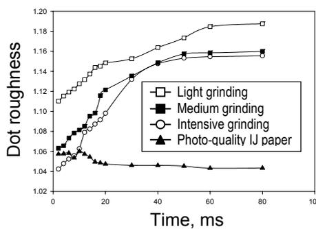
Fig. 3 Ink dot roughness changes with time for trial ink-jet papers coated with calcium carbonate ground at three levels
