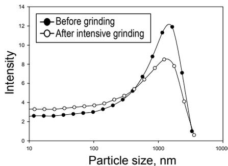
Fig. 1 Particle size distribution of calcium carbonate before and after grinding
