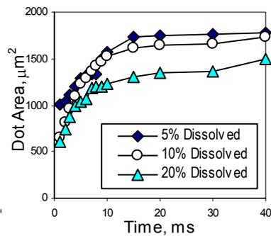
Fig. 4 Dot area changes with time for trial ink-jet papers coated with calcium carbonate dissolved partially with hydrochloric acid
