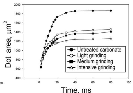
Fig. 2 Dot area changes with time for trial ink-jet papers coated with calcium carbonate ground at three
