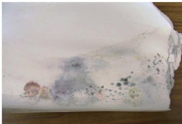
Photo. 2 Tsunami-damaged Uncoated paper left outside Hachinohe mill for 3 months.
