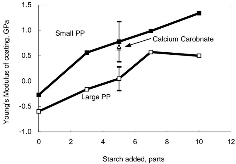
Fig. 7 Starch and plastic pigment(PP) effect on coating modulus.
