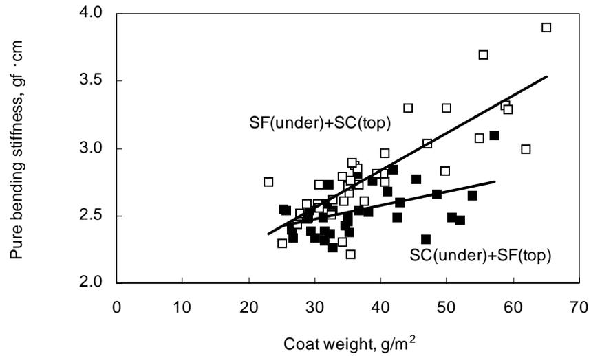
Fig.9 Effect of double-coating order of starch-containing(SC) and starch-free(SF) colors on pure bending stiffness of coated film.
