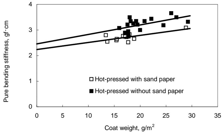
Fig. 5 Influence of interface shape on relationship between basis weight of coated film and pure bending stiffness.
