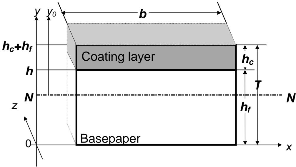
Fig. 1. Schematic cross section of coated paper for calculating second moment of area.
