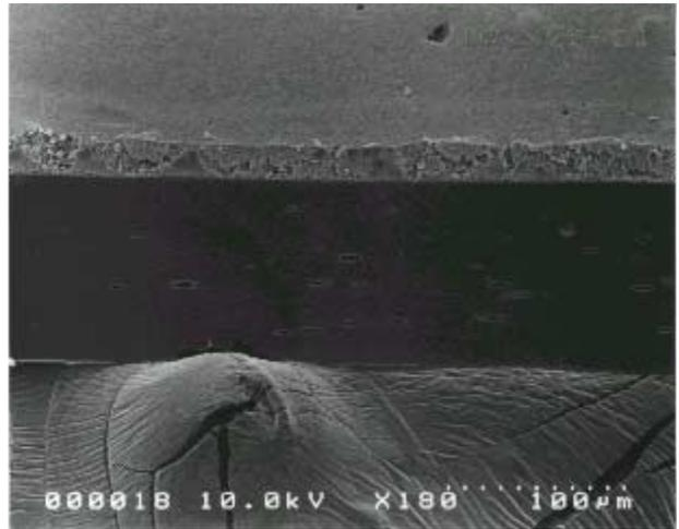
Picture 2. Cross section of coated film.
