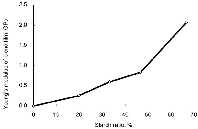
Fig. 6 Stach effect on modulus of latex/starch blend film
