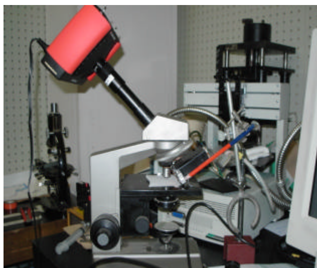
Photo 1 Ink-jet printing device with high-speed camera and microscope
