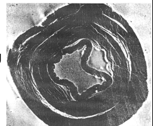
Lamellar separation of fiber cell wall by beating
