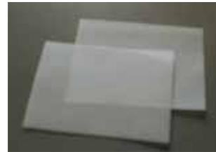
To figure out output characteristics, a standard film called Density Step Tablet was used. This tablet is a film consisting of portions at several different densities calibrated in a standard manner.
